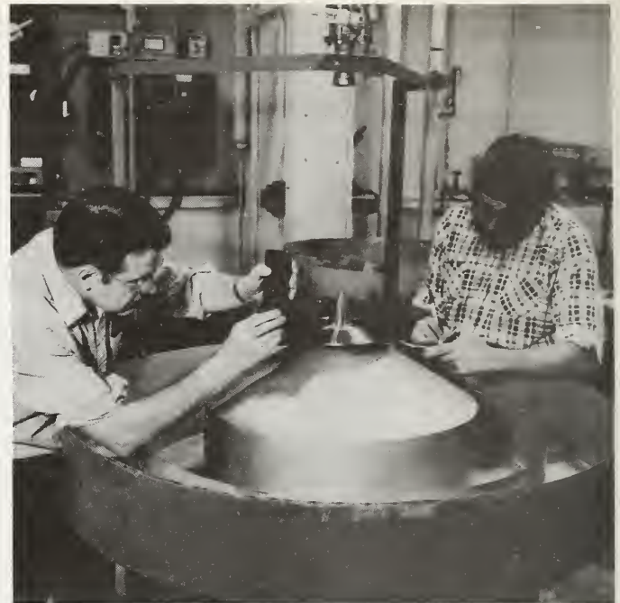
An experimental spinning disk separator takes a stream of recycled paper slurry and spins sticky contaminants to an outer ring while dropping useable pulp fiber to an inner ring. (Credit: USDA Forest Products Laboratory)
